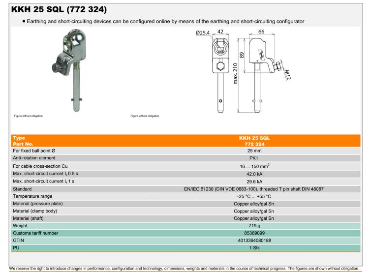
The clamps must be designed for the same maximum short-circuit current as the earthing and short-circuiting cables!
