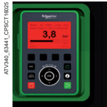
Detected fault: The screen's red backlight is activated automatically
