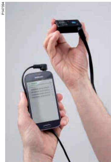
Each luminaire communicates with your Smartphone + VLDP probe
