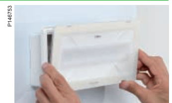
The body can be pre-installed. Just insert the cable through the cable gland, insert the wires into the screwless connector and just click the reflector into place.
