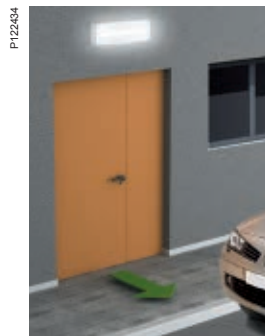
Near and immediately each outside exit.
