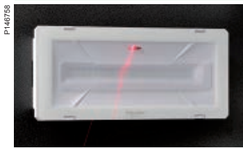
Product installed at a height? Laser beam to launch the test. Result on led and sent to the TBS.
