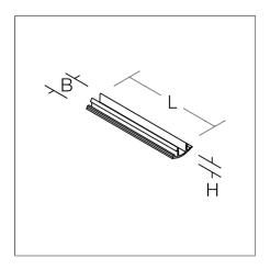
Plastic, cover for busbar, length 1 m, can be shortened as required. For 3-phase busbars and for RZB 3-phase DALI busbar.
