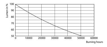
Lumen Maintenance Diagram - MAS LED spot VLE D 6.2-80W GU10 930 36D
