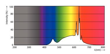
Spectral Power Distribution Colour - MAS LED spot VLE D 6.2-80W GU10 930 36D
