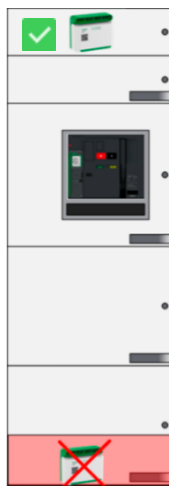
Illustration 3: HeatTag must be installed at the top of the cable compartment for feeder
