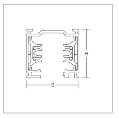
Aluminium extrusion profile painted, tracks can be cut to any required length, may be used within hand's reach, with five mounting holes at 100, 990, 1990, 2990, 3870mm.
