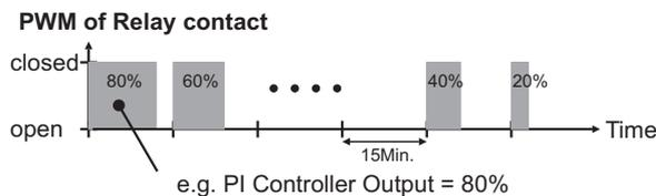
The parameter adjustments of the PI-controller (P), amplification P-band (I), re-adjustment time (Tn) can be changed by selecting the parameters 10, 11, 12.
