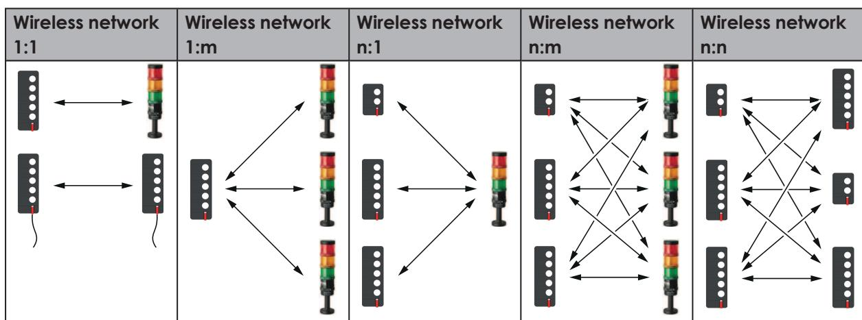
Andon WirelessBOXes with 2 or 5 buttons can be used together in a wireless network. The Andon WirelessBOXes can also have different button configurations.
