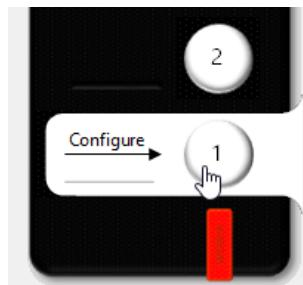
2. For each tier of the signal tower, select the status after pressing the button briefly (**short press**) and after pressing the button for longer (**long press**).
