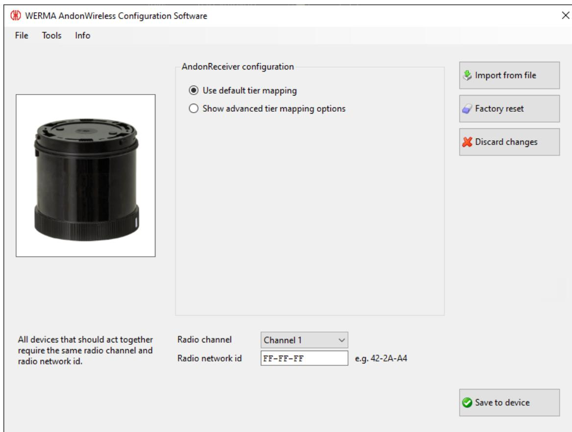
3. Click on **Save to device** to transfer the configuration to the Transceiver.
