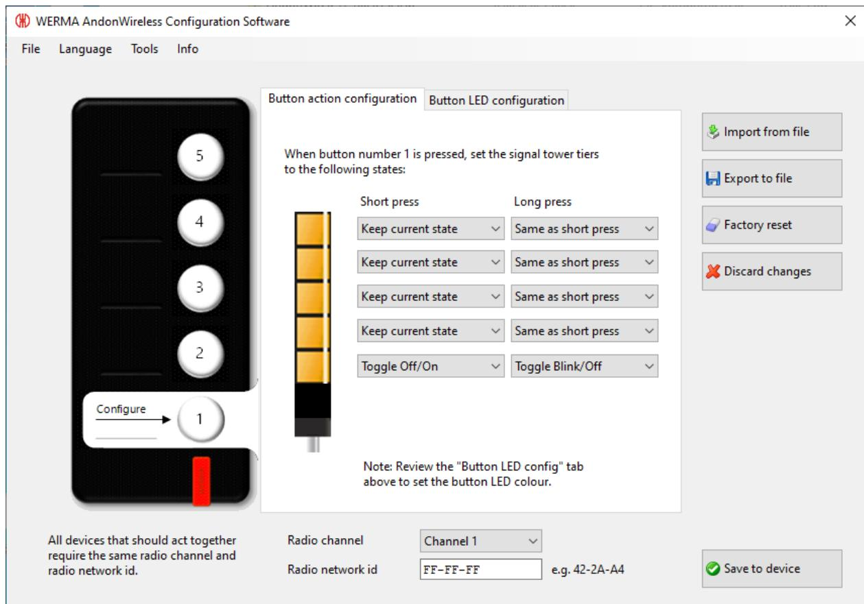
3. Click on **Save to device** to transfer the configuration to the Andon WirelessBOX.
