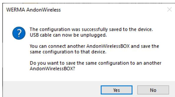
4. Click on **Yes** to transfer the current configuration to other Andon WirelessBOXes, see "Transferring the configuration to other Andon WirelessBOXes", S. 60.
