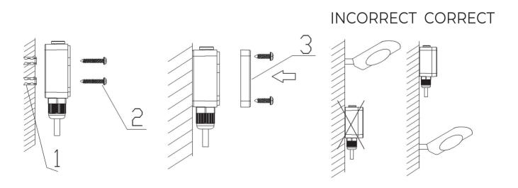
Install the product with the enclosed inflated screws. (See the figure on the right).
