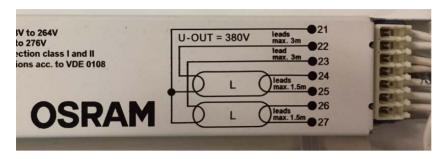
Step 2: Connect second fuse line to line "24" and "26"
