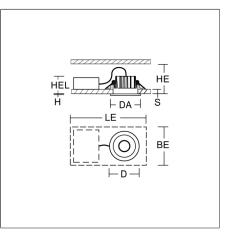
Round emergency luminaire for escape route lighting. With plastic lenses for area lighting. Suitable for connection to central battery systems. With AC Control monitoring module for LUXIFAIR central battery units. With enclosed separate ceiling mounting ring also suitable for ceiling cut-outs of Ø 68 mm.
