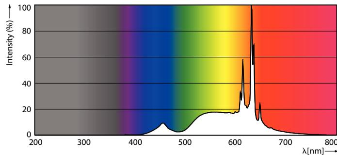
Spectral Power Distribution Colour - MAS LEDBulbDT10.5-100W E27 927A60CLG
