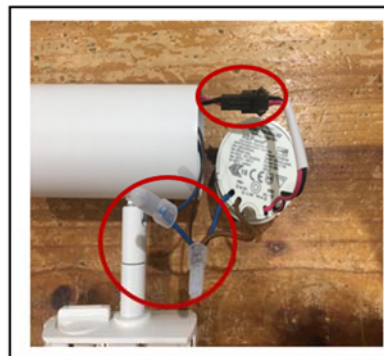
Figure2 Loose the connection
