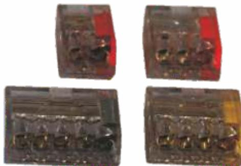
product description: quick and safe installation without screws, installation only by pushing terminals are intended for full Cu conductors for wires with cross-section from 1,0-2,5 mm<sup>2</sup> maximum working load of 24 A for voltages of up to 450 V transparent color for the visible control color-coding stripe
