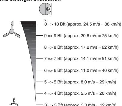
Position 3 - 0 defines the wind strength at which the blinds are raised.
