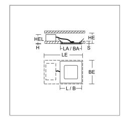
Square recessed downlight. For escape route illumination. Housing: die-cast aluminium, powder-coated. Lightguide and diffuser made of nonyellowing plastic (PMMA). Diffuser opal matt plastic. Ceiling installation with spring system. Including separate LED converter with connecting cable 250 mm. Suitable for connection to central battery systems. External driver with simple plug-in locking system.
